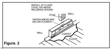
**NOTE:** Make sure the caution label with the word "TOP" is at the top of the heater. For most efficient operation locate heaters along outside wall under windows. Position heater so it can be secured to wall stud. Power cable must enter heater through one of the knockouts provided in wiring compartment. See Figure 3.
