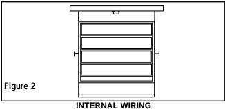
1. Heaters drawing 48 amps or more have internal subdivided branch circuit fusing.
