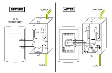
**Note 1:** All cables and connections must conform to the local electrical code. **WARNING:** Special CO/ALR solderless connectors must be used when connecting with aluminum conductors.
