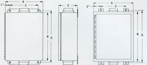
Weatherproof Sheet Steel Multi-circuit box protects thermocouple and instrument cables from corrosive or dirty environments.
